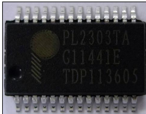
Figure 12-1 Chip Part Number Information
